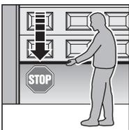
Demonstrate and test the safety return and the mechanical release. Only ever operate the door provided the door's range of travel is located within your field of vision.
